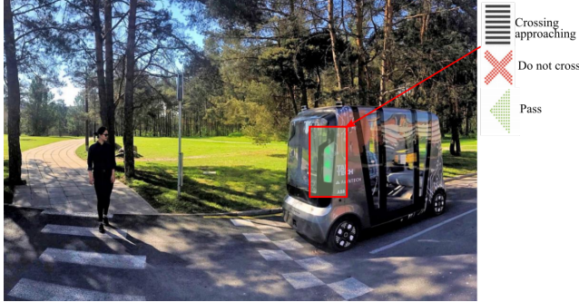
Figure 1: ISEAUTO shuttle signalling to the passenger that a pedestrian is detected, and it is safe to cross the road.
